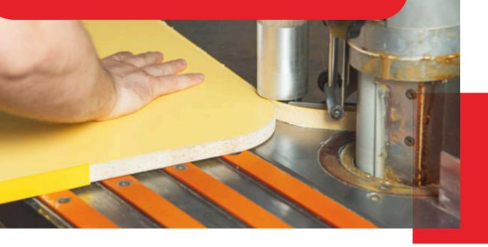
Free Bird Adhesives offers two primary options for manual edge banding: **828J** and **8062A**, available in natural **white** and yellow **transparent** colors. Both are specifically formulated for manual operations, featuring a low process temperature range of **120–150°C**, excellent bonding performance, high yield, and competitive pricing.
