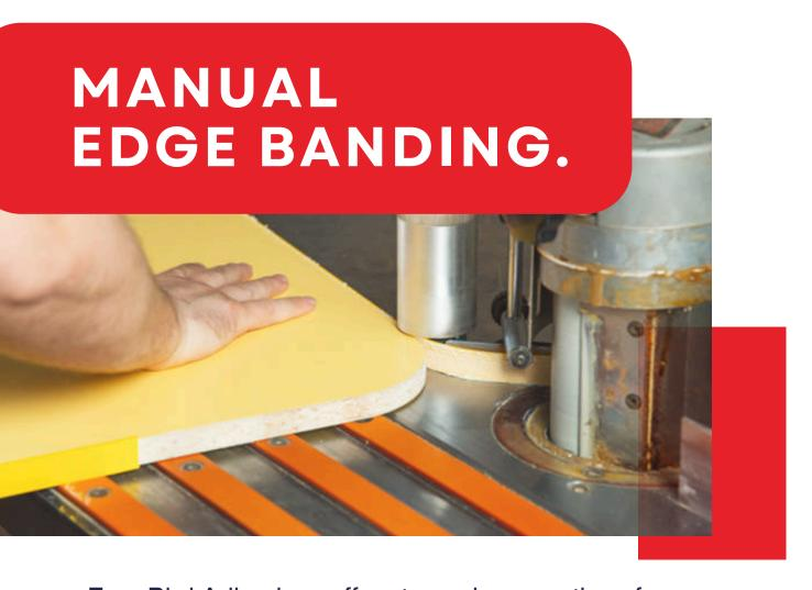
Free Bird Adhesives offers two primary options for manual edge banding: **828J** and **8062A**, available in natural **white** and yellow **transparent** colors. Both are specifically formulated for manual operations, featuring a low process temperature range of **120–150°C**, excellent bonding performance, high yield, and competitive pricing.
