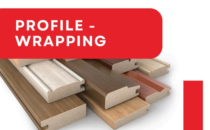
Free Bird Adhesives offers **8630A**, a primary EVA-based product, and **873N**, a polyolefin-based product, designed for wrapping profiles and frames made of <u>solid wood</u>, <u>particleboard</u>, and MDF with decor <u>paper</u>, <u>veneer</u>, and <u>CPL</u>. These adhesives provide superior bonding performance with good heat (UV-cured) and solvent (coating) resistance.
