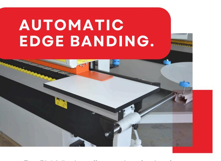
Free Bird Adhesives offers a variety of options for automatic edge banding, including featured choices of **826L** and **812S** for **high-speed** machines (180–210°C), and **858L** for **medium-to-slow-speed** machines (150–180°C). These options provide excellent bonding capabilities, high bond yield, and competitive pricing.
