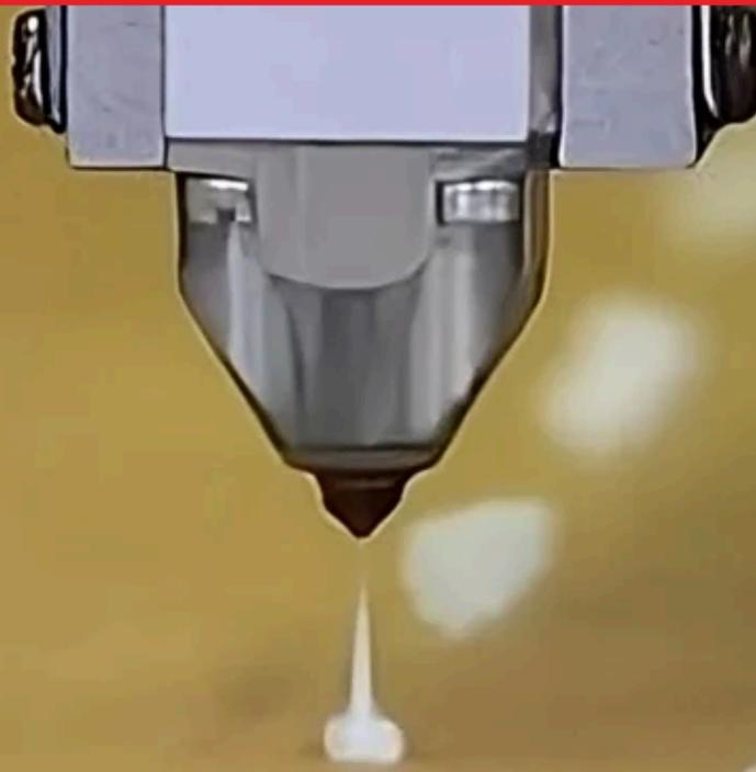
Hot melt adhesive is an ideal solution for bonding purposes in packaging processes. Its quick setting time and strong bonding capabilities, making it ideal for automated packaging lines.
