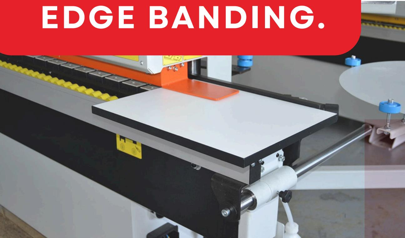
Free Bird Adhesives offers a variety of options for automatic edge banding, including featured choices of **826L** and **812S** for **high-speed** machines (180–210°C), and **858L** for **medium-to-slow-speed** machines (150–180°C). These options provide excellent bonding capabilities, high bond yield, and competitive pricing.
