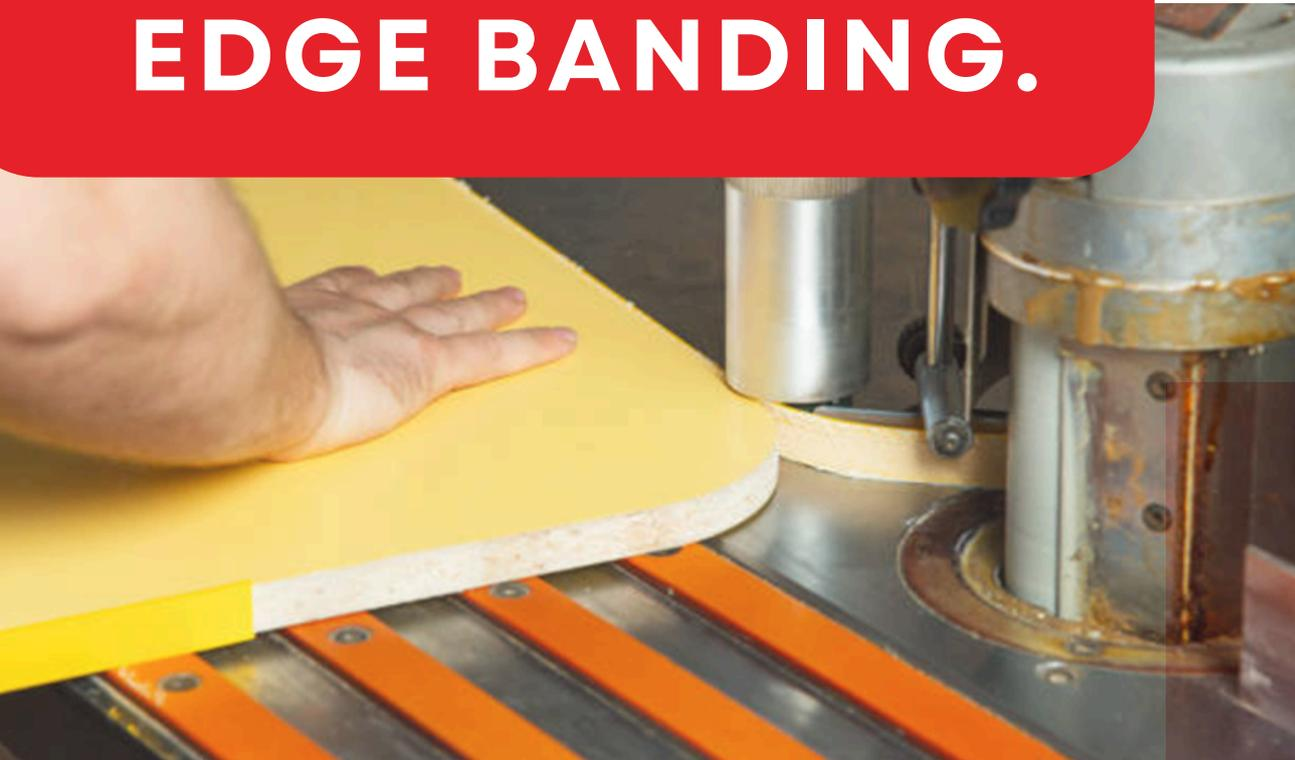
Free Bird Adhesives offers two primary options for manual edge banding: **828J** and **8062A**, available in natural **white** and yellow **transparent** colors. Both are specifically formulated for manual operations, featuring a low process temperature range of **120–150°C**, excellent bonding performance, high yield, and competitive pricing.
